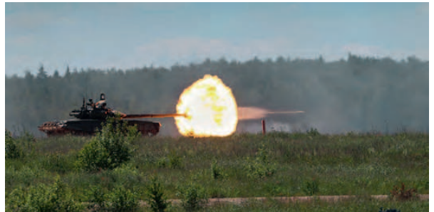
The firing of a shell causes a strong blast and a deafening noise around the tank. In front, the risks are considerable: ejection of the sabot, flames, strong shock wave...
